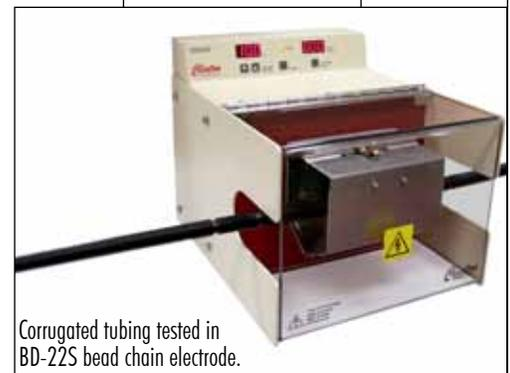
Corrugated tubing tested in BD-22S bead chain electrode.
