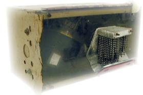
**6. Stabilize your wire as it runs through the electrode.** Some products, especially smaller wire running at very high speeds, are prone to an almost invisible lateral vibration that can cause false counting. A series of wire guides positioned before and after the electrode can reduce or eliminate problematic vibration.
